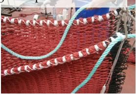
The codend is produced with an extra mesh and a half in spun dyed black nylon to close the codend & join it to extension
